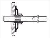
This device is situated inside the gearbox and is particularly recommended when gearbox protection is required in the event of accidental overloading. In this system, the final gear is connected to the gearbox output shaft by means of a friction assembly.
